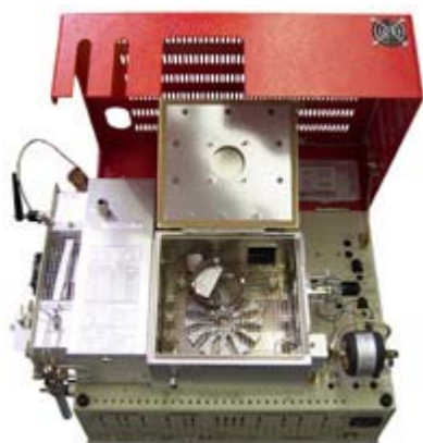
This Environmental GC is customized with a Thermal Desorber.
